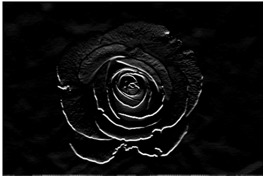
Figure 12: G_y convolution showcasing the edges in the vertical direction
