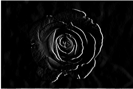
Figure 11: G_x convolution showcasing the edges in the horizontal direction
